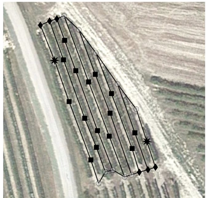
Fig. 4. Undirected graph that represents the available paths for the UGV on a real vineyard. Nodes are marked as described in Fig. 3 and represent the type A, B, AB nodes with the addition of some “transit” nodes marked as empty circles.
