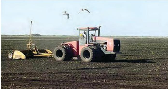
Figure 1. Land-leveling reduces sheet erosion and improves water management.
